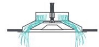
Figure 2. Air supply, heating.
